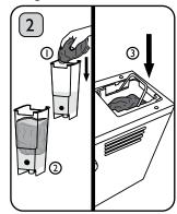
Fill Water Tank halfway (425ml). Place a tea towel in a plastic bag & place it in the Water Tank (1), above the water level to create a tight fit in the Water Tank (2). Place the Water Tank back inside the machine (3).
