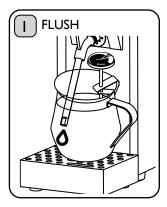
Flush the Steam Wand by dispensing steam to remove any milk residue from inside the Steam Wand after each use.
