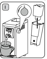
Ensure the Steam Valve is at 0. Turn on by pressing the ON/OFF Switch. Position the Milk Jug below the Steam Nozzle, remove Water Tank, then the Water Filter Holder & set the Water Filter Holder aside.
