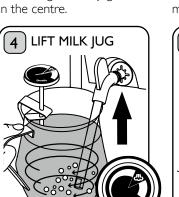
Once there is sufficient milk textured, raise the jug and continue until the Steam symbol is reached on the Thermometer Dial.
