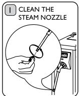
Unscrew the Steam Nozzle anti-clockwise and use a pin to remove dried milk. If too tight to unscrew, use an 8mm spanner. Screw Steam Nozzle back onto the steam wand, ensuring it is tight.
