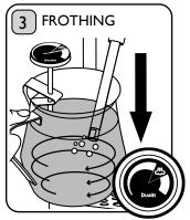
As the thermometer dial starts to rise, lower the Jug to bring the Nozzle to the surface of the milk. This will start to introduce air and develop the froth. Large bubbles indicate nozzle is raised too high.
