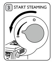
Slowly open the Steam Valve to halfway. Pump will start and steam will flow from the Steam Wand Nozzle. To speed up the process, gradually open the Steam Valve, take care not to splash milk.
