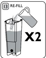
Open Steam Valve and allow all the water in the Water Tank to dispense into the container. Re-fill Water Tank with fresh water and repeat. This will remove any traces of the descale solution within the machine's internals.
