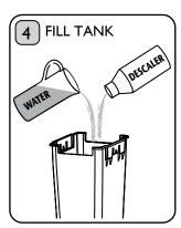
Fill Water Tank with 1 litre of Descaler Solution. Follow instructions & safety precautions on the Descaler packaging; Dualit recommends using Kilrock Espresso & Coffee Machine Descaler. If using granular descaler, ensure it is fully dissolved before switching the machine on.
