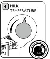
Warning: Never lift the Steam Wand Nozzle out of the milk whilst Steam Valve is open. The Steam symbol on the Thermometer indicates recommended milk temperature. When desired milk temperature is reached, close the Steam Valve.
