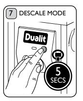
To enter the Descale Mode; Press and hold the Descale Button for **5 seconds**. Once released the Indicator Light will quickly flash red to indicate machine is in Descale Mode.
