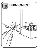
If the machine is accidentally switched off whilst in Descale Mode, switch back on, the machine will automatically enter back in Descale Mode. Continue process.
