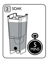
Soak for 5 minutes to activate the Water Filter. Discard the water. The Water Filter only needs to be activated before first use. From then on, you can fill the Water Tank as normal.
