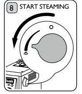
Open Steam Valve; steam will dispense initially, followed by Descaling solution. Dispense all solution. Indicator Light will flash Red and Amber when Water Tank is empty.
