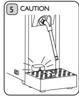
CAUTION: HOT / RISK OF SCALDING. Keep hands away from the Outlet at all times. Some steam and water will expel into the Drip Tray from the Outlet when the Steam Valve has just been closed. This is normal operation.
