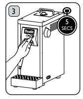
Press & hold the Descale Button for 5 seconds. The Indicator Light will flash red.
