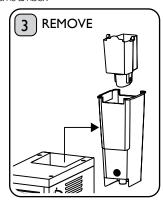
CAUTION: Remove Water Tank from machine then remove Water Filter Holder from Water Tank. Do not allow Descale Solution to come in contact with Dualit Water Filter. Risk of injury or contamination!
