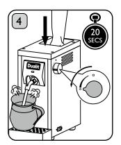
Turn the Steam Valve fully anti-clockwise. Gently apply downward pressure to the plastic bag; until water comes out of the Steam Nozzle. Note this may take up to 20 seconds. **Caution: Steam**
