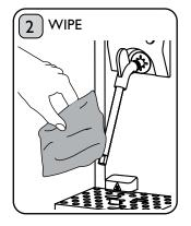
Thoroughly wipe the Steam Wand to clean off any milk residue with a damp cloth. CAUTION: Steam Wand will be hot.
