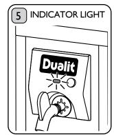
The Indicator Light will flash Green whilst warming and stop flashing when ready to use. If it's Amber or Red, see Quick Reference Guide on page 09.
