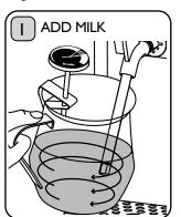
Add milk to the jug. Holding the Jug by the handle, and at a slight angle, place the tip of the Steam Wand Nozzle I-2 cm below the surface. The wand should be close to the edge of the jug, not in the centre.
